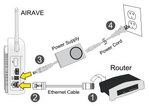
8. Insert one end of the power cord into the power supply and then plug the other end into an available power outlet (4).
