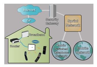
About the size of a traditional wireless access point (WAP), the base station pipes voice and data through the Internet to the Sprint network, which then routes the signal to the desired party on either the Public Switched Telephone Network (PSTN) or Mobile Network.
