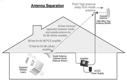
Connect the outside antenna to the amplifier with Wilson 400 low loss coax cable (available from Wilson Electronics). Place the inside antenna in the center of the area needing the amplified signal. It is important to have at least 50 feet of separation between the inside and outside antennas for the 50 dB amplifiers, 68 feet of separation distance for the 60 dB PCS amplifiers and at least 75 feet of separation distance for the 60 dB cellular amplifiers.
