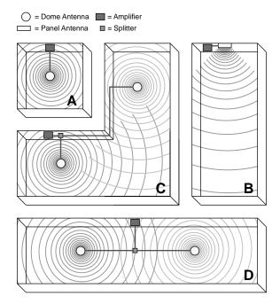
Connect the coax cable from the amplifier to the inside antenna. For distances of 20 feet or more, use Wilson 400 low loss coax cable to prevent significant signal loss.
