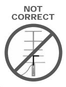
Warning: The outside antenna must be installed on an outdoor permanent structure with a separation of at least 20 feet from all persons during normal operation.
