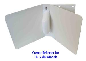
Mobile Mark's high frequency Corner Reflector antennas are useful for applications such as surveillance work, 1.8/1.9 GHz GSM, and other high frequency applications.
