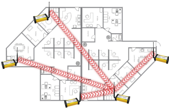
EXAMPLE 1 Indoor point-to-multipoint wireless Ethernet system
