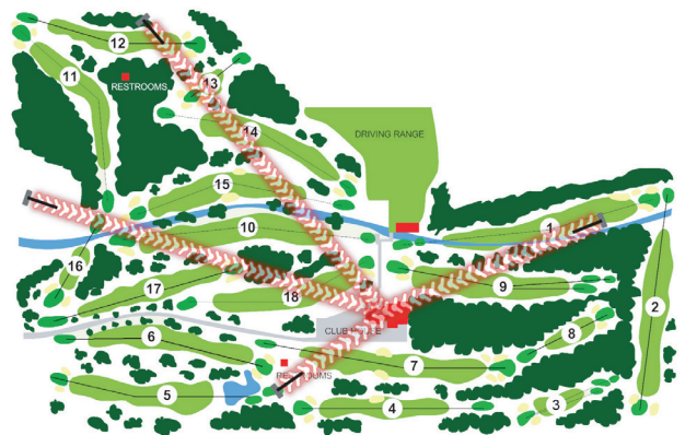
EXAMPLE 2 Ultra-long-range, point-to-multipoint wireless system transmitting Ethernet data across golf course
