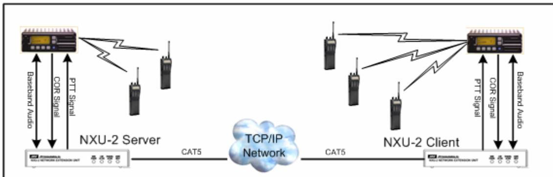
When the mobile or portable LMR users in the field transmit to the Server radio (left), their program audio will be transmitted by the Client radio (right) at the far-end NXU-2 RoIP link. LMR users at both ends of the link will be able to 'virtually' communicate with each other by utilizing the NXU-2 link created over the TCP/IP network.
