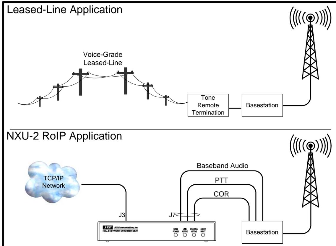
Two NXU-2's can be associated across a TCP/IP network by assigning one NXU-2 as a *Server*, and the other NXU-2 as a *Client*. The purpose the *Server NXU* is to wait on the network for a *Client NXU* to connect to it. The purpose of the *Client NXU* is to locate and connect to as specific *Server NXU* over the network. Once the association is established (typically within 5 seconds) RoIP traffic can commence in full duplex fashion.
