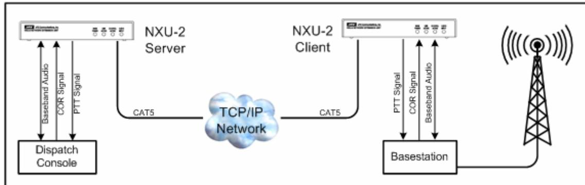
The previous example illustrates the original example of a typical leased line dedicated link between a dispatch console and a remote basestation, except (2) NXU-2 Network Extension Units linked together using an existing TCP/IP network are used at each endpoint to support the dispatch console and the basestation, thus eliminating the leased line.
