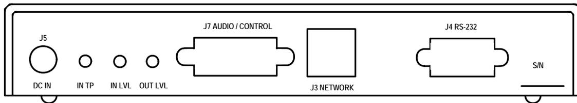
Any of the ACU® Radio Interface Cables manufactured by JPS Communications can be used to interface a radio to the NXU-2 unit. However, the supplied crossover adapter must be inserted between the NXU-2 J7 connector and the JPS Built Radio Interface Cable to “Crossover” the proper control signals. Naturally, the end-user can fabricate similar cables and connect the leads to the associated pin on connector J7, thus eliminating the need to use the Crossover Adapter.
